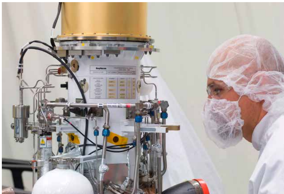
In Raytheon's Space Factory in Tucson, Arizona, a technician inspects an exo-atmospheric kill vehicle, which travels through space to track and attack enemy missiles.
